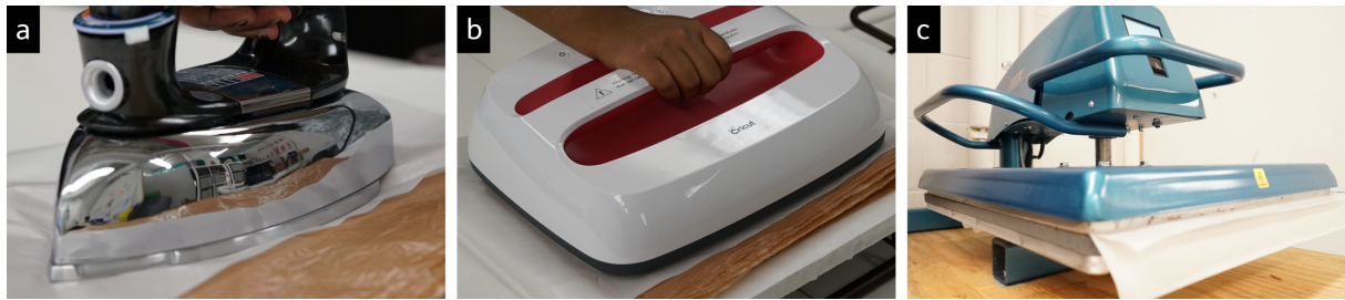
Figure 3. Different tools for global fusion: (a) a clothing iron: Black + Decker "The Classic" model, (b) a handheld heatpress: Cricut EasyPress, and (c) a tabletop heatpress: HIX Swingman 20.
