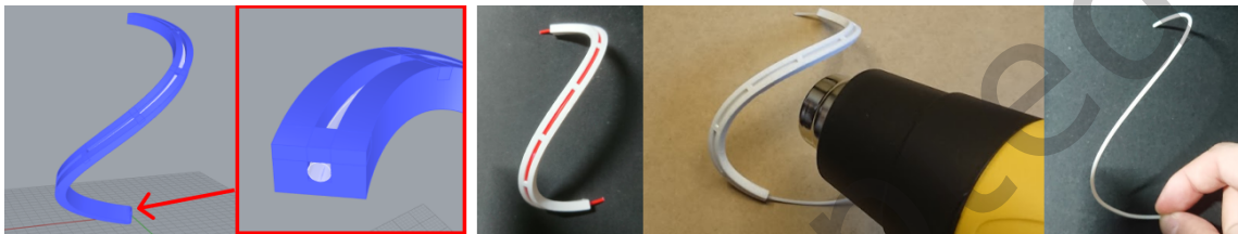
Fig. 14. By applying heat to the filament inserted into the proxy and cooling it, we can reshape the filament.
