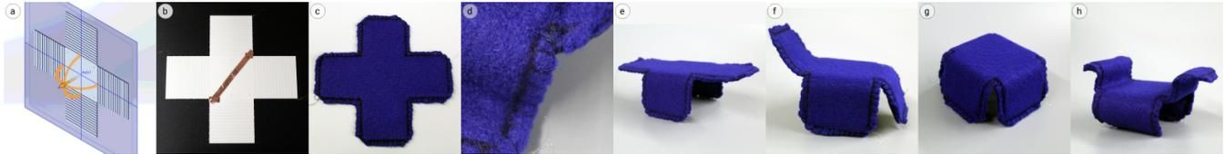
**Figure 7: Multi-Purpose Seating (scale model):** (a) Section view of the seating panel (b-d) Assembling the circuit and stitching on felt. Use of localised shape forming to create (e) cot, (f) recliner chair, (g) stool, and (h) window seat
