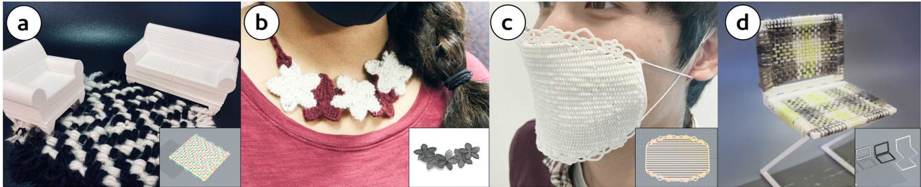
**Figure 1:** EscapeLoom is a computational design tool to afford new weaving workflows for novice users: Weaving a rug in complex pattern using a water-soluble guide (a), 3D printing custom shaped looms in flexible material to form a necklace and a mask (b-c), and 3D printing a rigid geometry to construct global shape with soft woven parts like a chair (d).
